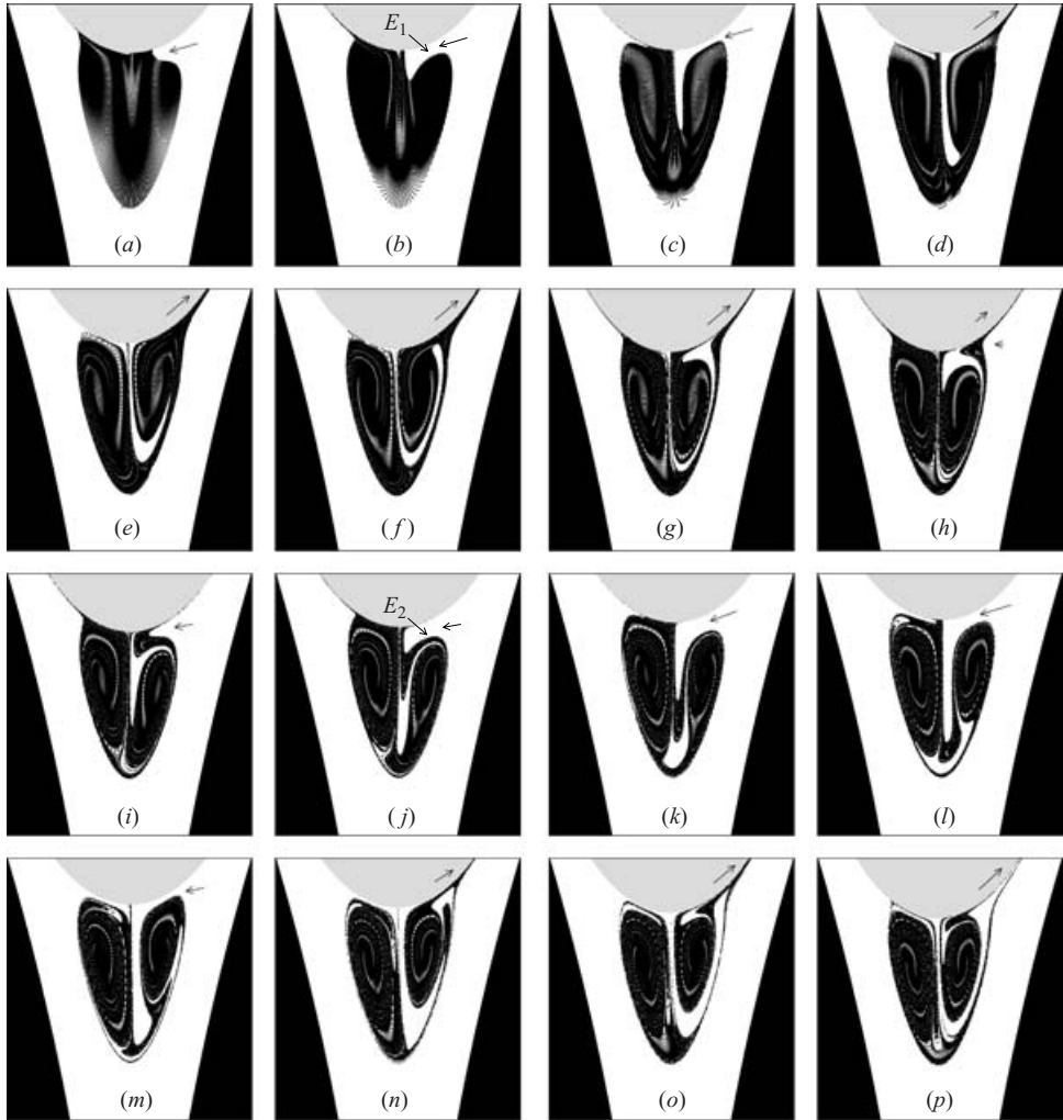
FIGURE 9. Numerical simulation of approximately 60 000 points initially uniformly spaced (via a square grid) within the steady-state (symmetric) recirculation zone corresponding to \bar{S} = 1 . The phase increases in steps of 0.1 from 0.275 at (a). The Hooke's joint angle was 30^\circ , giving S as in figure 7.
